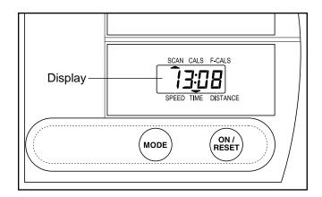
Speed—This mode displays your pedaling speed, in miles per hour.
